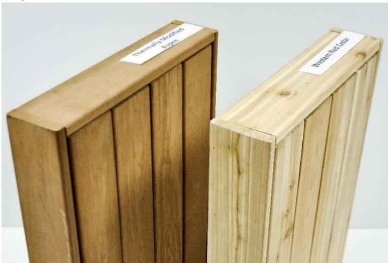
**Figure 1.** Decking samples of thermally modified aspen (left) and Western red cedar (right). Photo credit: Maria Fernanda Laguarda Mallo.
