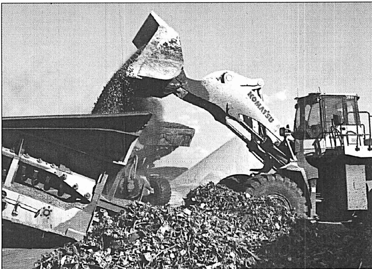
Workers shift taconite rock into a hopper from which it is fed by conveyor to the barge's hold. The rock will be shipped to Chicago for use in road construction. Bob King / rking@duluthnews.com
